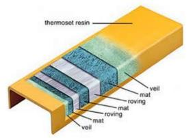
The above sketch and photo shows fibreglass strands and veil being pulled through the coloured resin mix as part of the FRP construction process.
