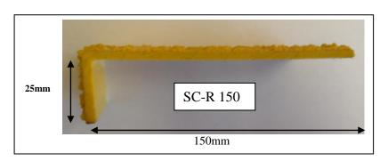
Staircare SC-R 150 have been designed to offer lasting slip resistance. They are made from a composite material that is suitable for use in harsh environments; including, high exposure to salt water. During the manufacture process silicon carbide is incorporated to form an inseparable gritted surface. SC-R 150 are available in yellow with UV protection and a heavy duty silicon carbide anti slip grit for serious slip protection.
