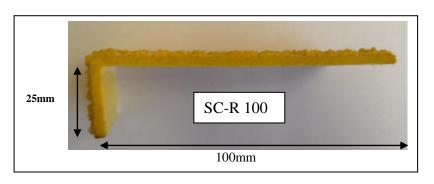
Staircare SC-R 100 have been designed to offer lasting slip resistance. They are made from a composite material that is suitable for use in harsh environments; including, high exposure to salt water. During the manufacture process silicon carbide is incorporated to form an inseparable gritted surface. SC-R 100 are available in yellow with UV protection and a heavy duty silicon carbide anti slip grit for serious slip protection.
