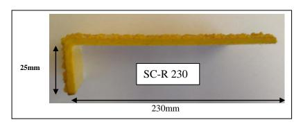
Staircare SC-R 230 have been designed to cover most of the step and offer lasting slip resistance. They are made from a composite material that is suitable for use in harsh environments; including, high exposure to salt water. During the manufacture process silicon carbide is incorporated to form an inseparable gritted surface. SC-R 230 are available in yellow with UV protection and a heavy duty silicon carbide anti slip grit for serious slip protection.
