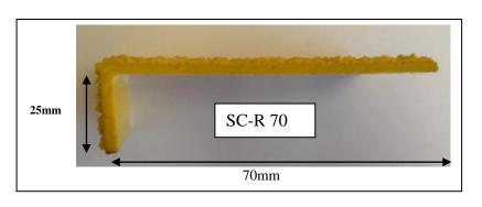
Staircare SC-R 70 have been designed to offer lasting slip resistance. They are made from a composite material that is suitable for use in harsh environments; including, high exposure to salt water. During the manufacture process silicon carbide is incorporated to form an inseparable gritted surface. SC-R 70 are available in yellow with UV protection and a heavy duty silicon carbide anti slip grit for serious slip protection.
